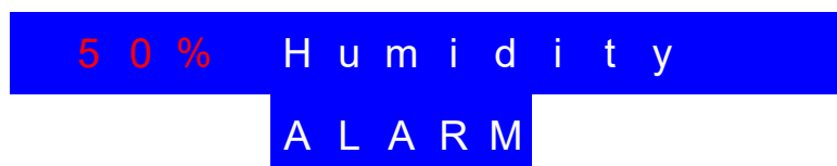
Fig. 20 - Display message for the humidity alarm. The digits highlighted in red blink. The words "Humidity" and "ALARM" light up rotationally.
