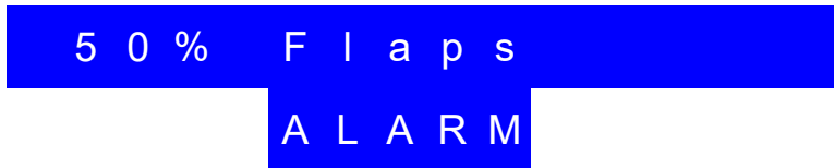
Fig. 21 - Display message for the flaps alarm. The words "Flaps" and "ALARM" light up rotationally.
