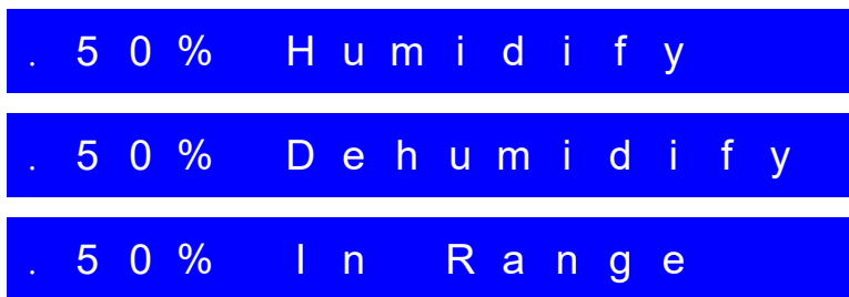
Fig. 7 - Possible display messages during normal operation (Slave sets).
